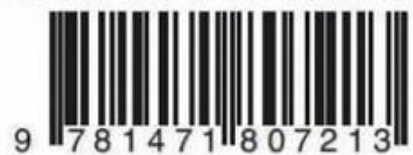
Figure 6.14 Barcodes are made up of alternating dark and light lines of varying thickness
